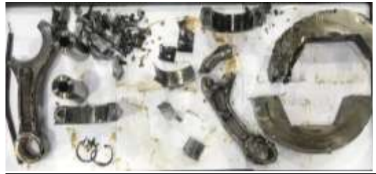
Engine part retrieved from oil pan
