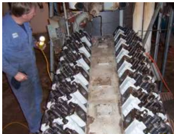
Inspecting recently installed refurbished cylinder heads
